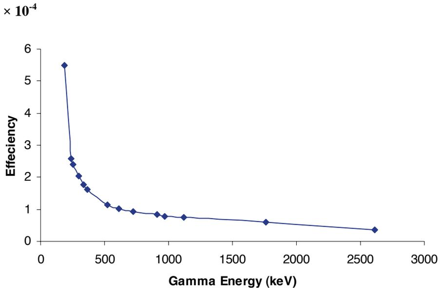
**Figure 2: The Photopeak Efficiency of HPGe detector**
