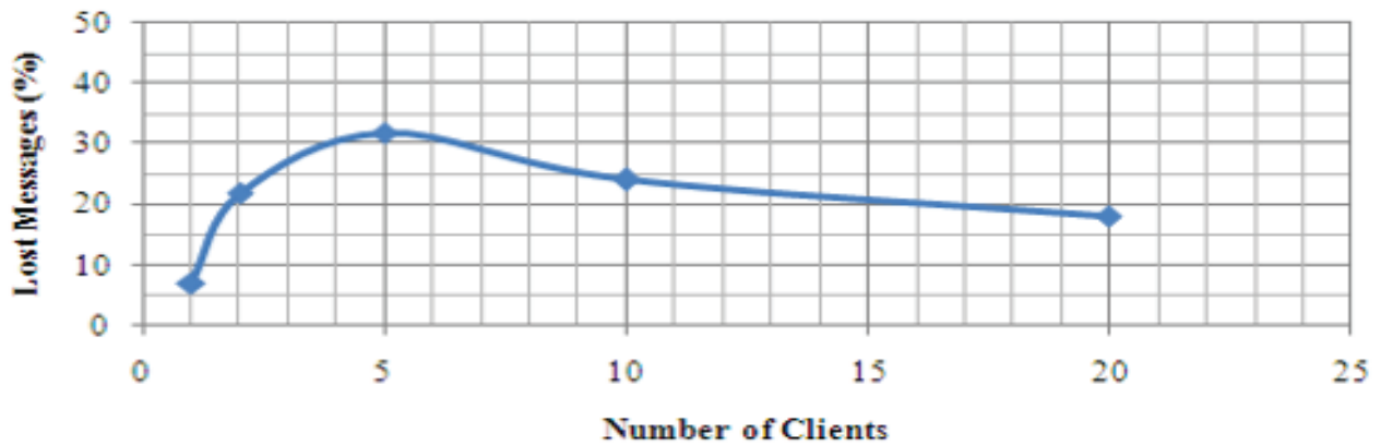
Fig 5 Lost messages of local commercial MQTT server
